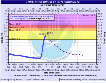
This graph from August 18, 2023 displays a sudden, dramatic stream-rise from just over 2 feet to over 10 feet within the space of a few hours overnight. Several inches of rain had fallen in the watershed onto soil that was already saturated from previous rain events.
